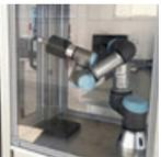
Automated spreading has been demonstrated as a key parameter for improving repeatability and reproducibility of the *in-vitro* UV tests compared to manual spreading. The HD-SPREADMASTER from HelioScreen is a robot which carries out the automatic spreading of the sunscreen on the substrate. It allows a total control of the product spreading and ensures the reproducibility of the *in-vitro* UV testing with a very low variability range. The specifications of this appliance are
