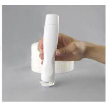
Step 4: Wait another 30 seconds. Then use a dry cellulous swab to thoroughly dry the probe surface. Do not hold the probes with the measurement surface pointing upwards before it is dry, to prevent the liquid from entering the probe electronics.
