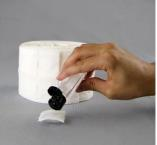
Step 3: Press the probe onto the wet swab and hold it pressed for approx. 10 seconds, then take off the probe.
