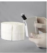
You may also use a swab with Zanitize to clean the outside of the cartridge and the light diode inside the tube on the device. Dry the inside of the tube it with another swab before using it again.
