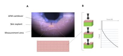
A: The AFM tip is positioned on the explant and a matrix of force-indentation curves is acquired.
